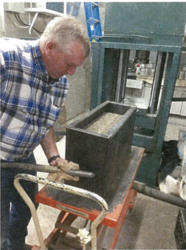
pea gravel consolidation being performed with an electric concrete vibrator
