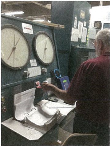
load rate being monitored
