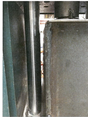
steel box beginning to bow
