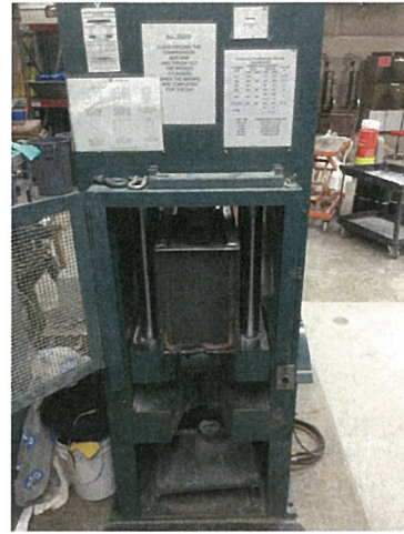
filled box within compression machine
