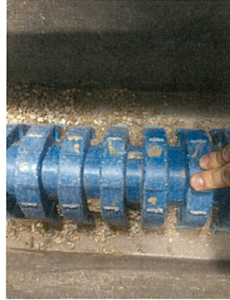
minor indentation found on top of device
