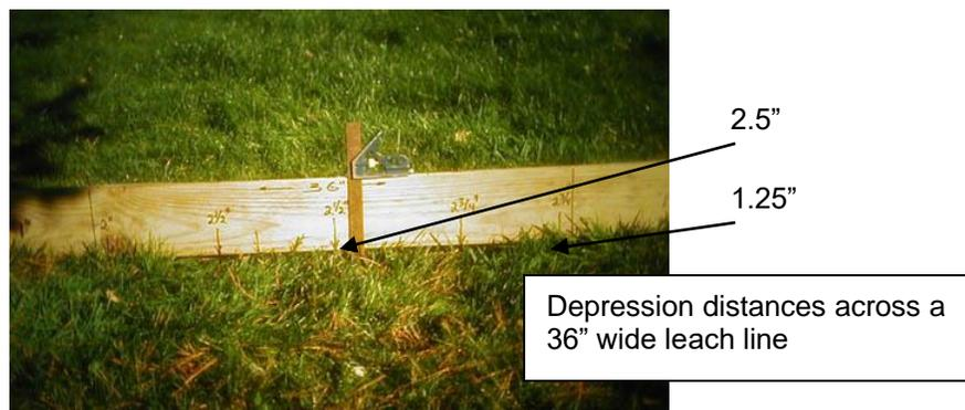
In addition to siltation, the traditional stone-fill leach lines present other inherent steady-state operational problems. Typically, the perforated leach line pipe is a four-inch (diameter) PVC pipe that passively delivers sewage effluent to the stone fill. The void spaces permit liquid sewage to flow throughout the field, and with no capillary action
