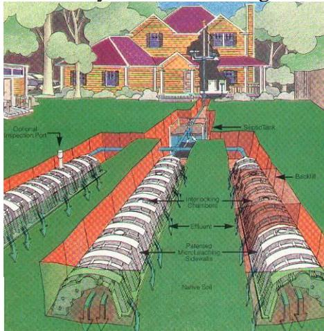
Few systems are total failures “at the starting block”, and most professional installers will warranty conventional systems for a year. **EPIC** systems are just better performers
