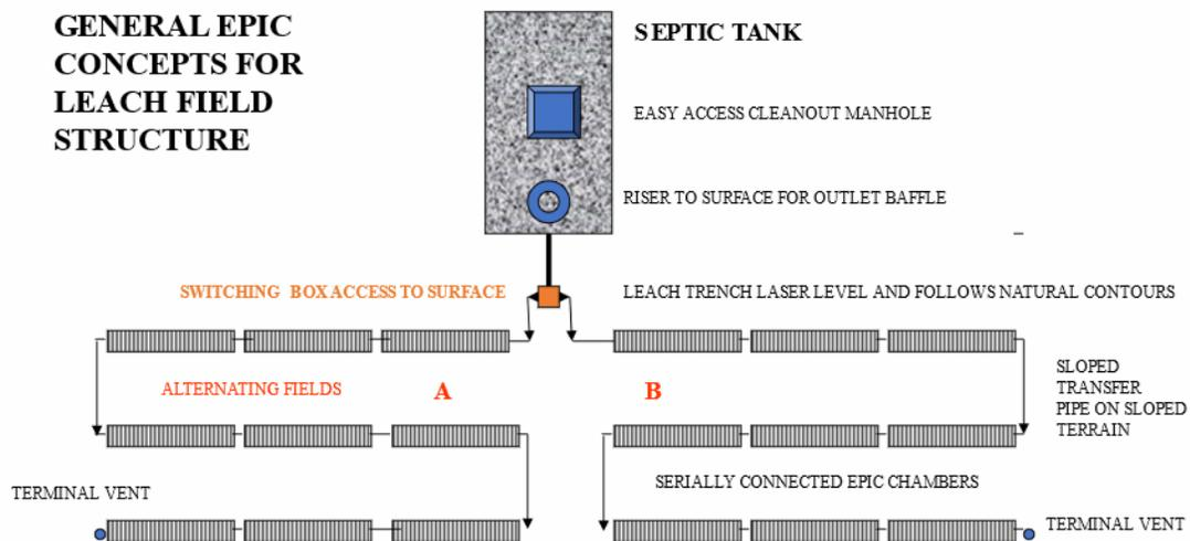
**FIELD SIZE DETERMINED BY COUNTY STANDARD APPLICATION RATES AND PERCOLATION DATA. RECOMMENDED FIELD AREA DIVIDED BY TWO INTO TWO DISTINCT ALTERNATING FIELDS. FIELDS ARE ALTERNATED ON A YEARLY BASIS THROUGH SWITCHING BOX OR VALVE. SLUDGE DEPTH IN SEPTIC TANK MEASURED ANNUALLY WHEN FIELD SWITCHING MADE. LINE SEPARATION 6'-10'(+) , BUT ACTUAL SEPARATION DETERMINED BY SLOPE OF LAND.**
