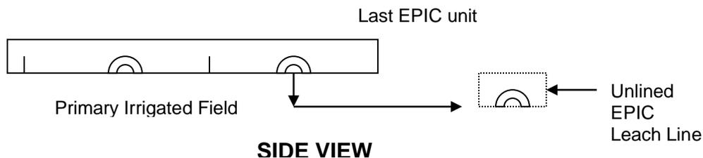
A simple addition of **40'** of leach line will provide a storage capacity of over **260** gallons of overflow capacity, which is then absorbed in the surrounding soil.
