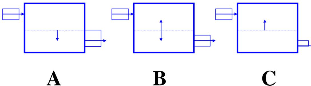
In **Figure C**, regardless of the volumetric capacity, the liquid level will rise since the outflow rate (as determined by the available openings) is smaller than the incoming flow. In **Figure B** the liquid level is stable because the inflow rate matches the outflow rate, and in **Figure A**, the liquid level drops quickly because the outflow exceeds the inflow rate.
