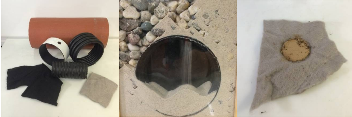
Common Drainage Pipe and Fabric
